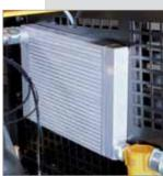
The compressed air is cooled to 7°C above ambient temperature. Accumulated condensate is able to drain away easily, as the compressed air cooler is installed at an angle, whilst the hot exhaust gasses from the motor are also used to aid condensate evaporation. This design consequently ensures reliable frost
